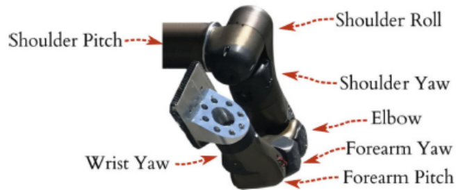
Figure 5.2: Centauro robot arm
